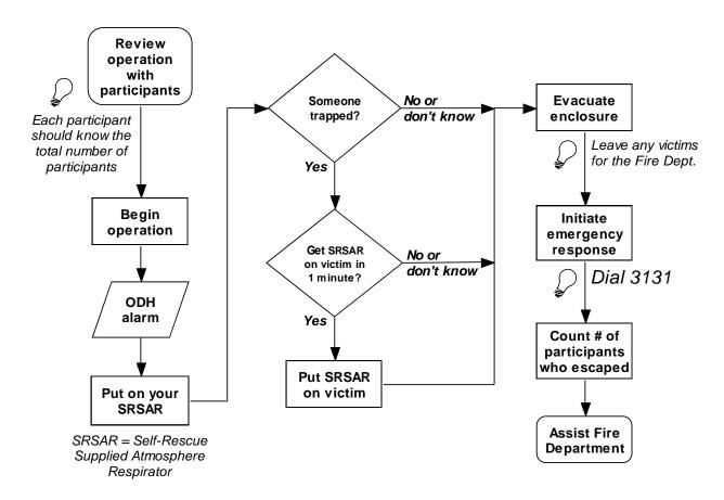
Figure 3 - Emergency evacuation and rescue flowchart
